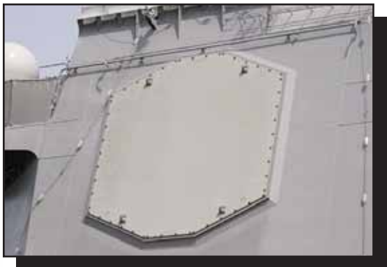
The AN/SPY-1D phased array radar
