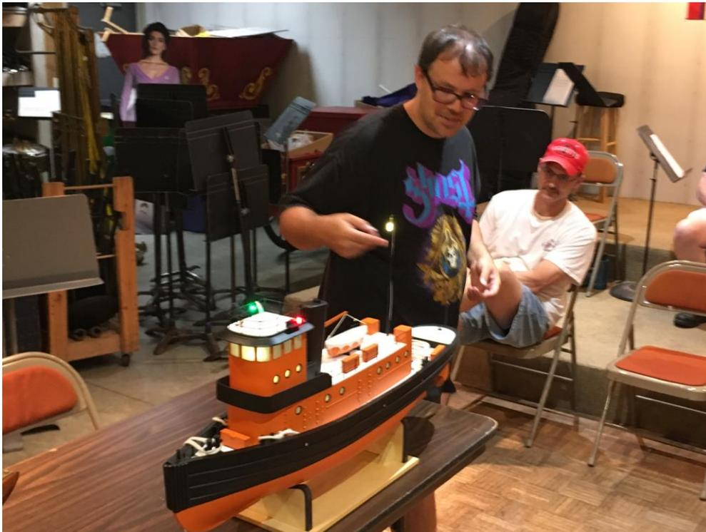
Looks a lot like a Brooklyn I think. A 12 volt system where the water that comes from the fire nozzle also cools the motor, it runs all the time. He has also fitted it with twin floating mesh bags to clean debris from the surface of the pond:
