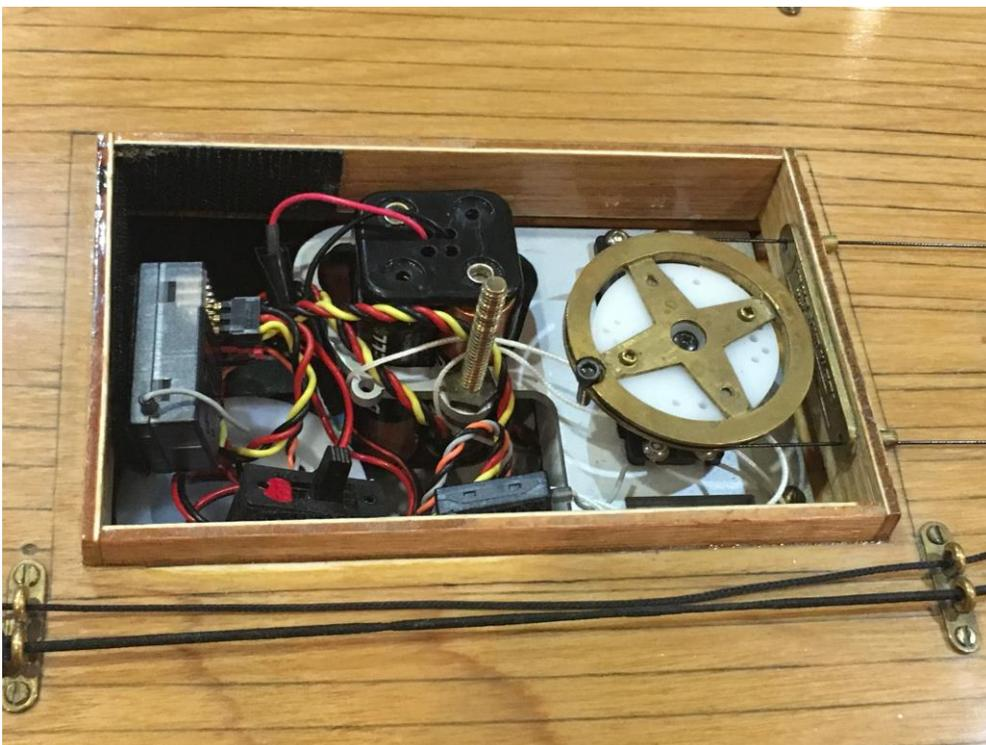
Tight access to the winch for the sails, the drum is below the wiring lower left in the opening. The wheel/pulley at the right is for the rudder.
